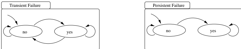
Fig. 7. Failure automata for transient and persistent failures
